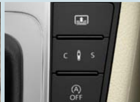
DCC, Dynamic Chassis Control
