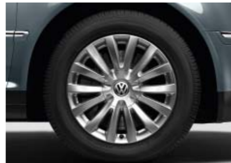
Four 7½ J x 17 “Impression” alloy wheels, size 235/55 R 17 H winter tyres in addition to the summer tyres selected.
