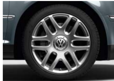
Four 8½ J x 19 "Helios" alloy wheels, 255/40 R 19 tyres, painted in Sterling Silver.
